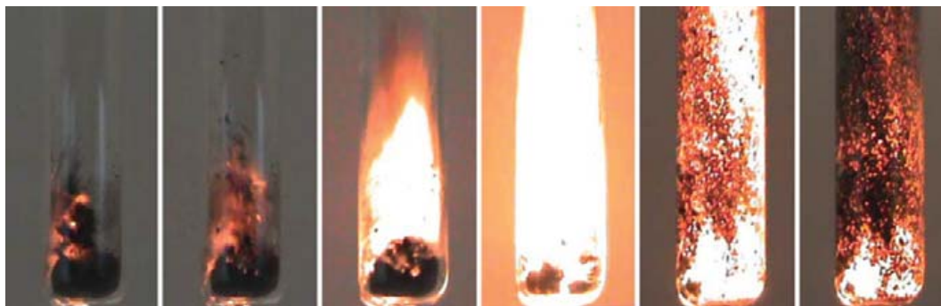
Figure 1 A sequence of photographs (0.04 s intervals) of the reaction of \text{NbCl}_5 with \text{Li}_3\text{N} in the SSM formation of \text{NbN} . The reaction was initiated through external heating using a hot plate. Reproduced from Meyer, H. -J. Dalton Trans. 2010 , 39, 5973, with permission from Royal Society of Chemistry.
